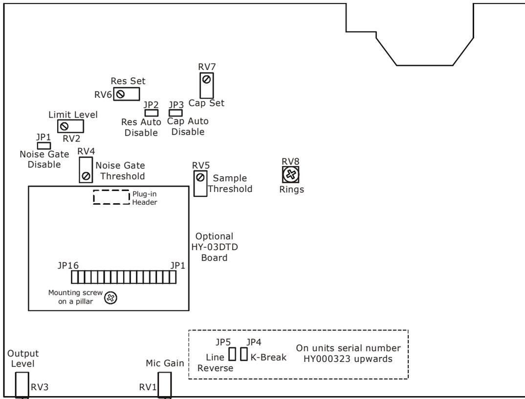
**Figure 1-3 : HY-03 Preset Controls and Alignments**
