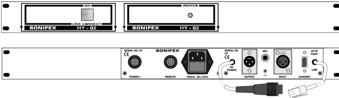
**HY-02T** Twin automatic TBU, rack mounted with PSU
