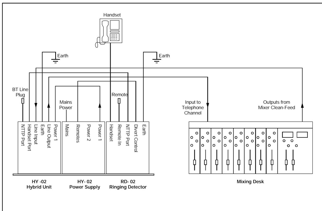
Connect the lead from the DIVERT CONTROL connector on the rear of the ring detector section to the REMOTES connector on the rear of the power supply. The NTPP port connection from the RD-02 should be connected to the HANDSET connector on the rear of the HY-02 unit. Make all the other connections as for a single HY-02.
