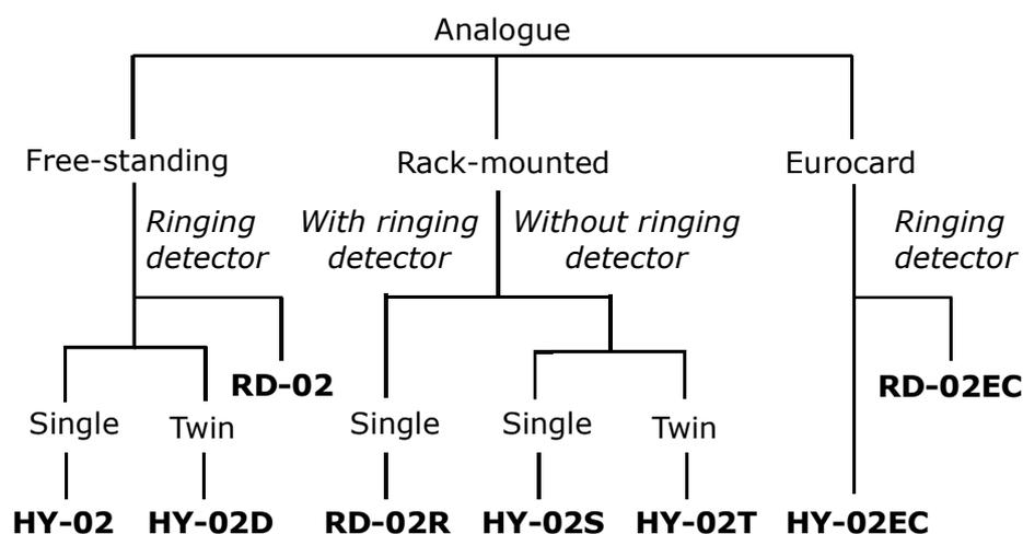
The HY-02 analogue telephone hybrids are available as free standing, or 1U 19" rack-mount units, supplied in either single or twin configurations. Each has a separate approved power supply. The hybrid can also be supplied as a single eurocard. Ringing detectors are available as a separate free standing unit, as a eurocard, or can be rack-mounted with a single HY-02 (the RD-02R).
