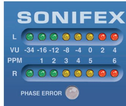
Fig 1-8: RM-CA2 & RM-CAD8 Meters & Phase Error LED
