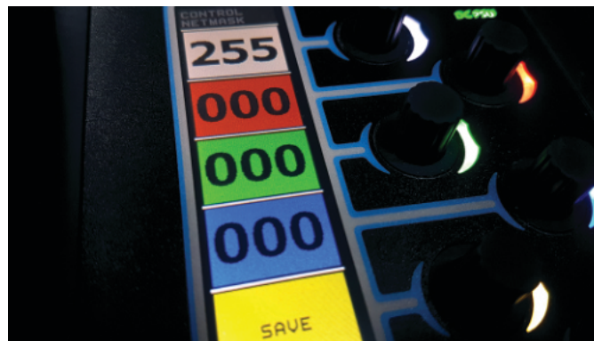
16. This takes you back to the control port sub-menu. Select 'Netmask' using the green encoder, and then change the subnet to match the subnet of your PC, again selecting 'Save' once complete.
