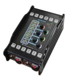
Dante AoIP input to any physical output or Dante output, you can define your own audio pathways. Additionally you can choose which of those pathways need to be controlled (volume and pan) by the use of rotary encoders.
