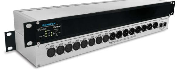
The AVN-AIO8R audio converter and interface converts up to eight analogue inputs and eight analogue outputs to and from the Dante Audio-over-IP networking standard. Dual Ethernet ports allow the unit to operate in redundant mode. ensuring audio routing is maintained in the event of loss of link on either of the network connections.
