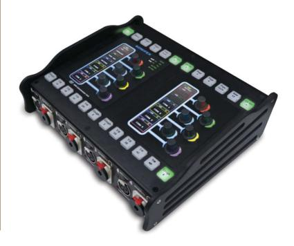
outputs or cross-points, allowing talkback feeds, commentary and audio mixing to be handled in one unit
