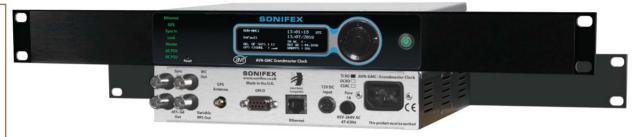
The AVN-GMCS is a PTPv2 grandmaster clock for use with AoIP applications. IEEE1588-2008 PTPv2 (precision time protocol) is used to synchronise all the nodes within a network. To achieve this one of the nodes must become the master clock and distribute time packets to the others. The AVN-GMCS is designed to perform this role simply and accurately, enabling sub micro second synchronisation between all nodes.
