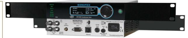
The AVN-GMCOS is a PTPv2 grandmaster clock for use with AoIP applications which uses a temperature controlled crystal for GPS holdover accuracy. IEEE1588-2008 PTPv2 (precision time protocol) is used to synchronise all the nodes within a network. To achieve this one of the nodes must become the master clock and distribute time packets to the others. The AVN-GMCOS is designed to perform this role simply and accurately, enabling sub micro second synchronisation between all nodes.
