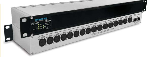
The AVN-AI16R audio converter and interface converts up to sixteen analogue inputs to the Dante Audio-over-IP networking standard. Dual Ethernet ports allow the unit to operate in redundant mode, ensuring audio routing is maintained in the event of loss of link on either of the network connections.
