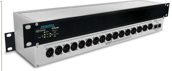
The AVN-AO16R audio converter and interface converts up to sixteen analogue outputs from the Dante Audio-over-IP networking standard. Dual Ethernet ports allow the unit to operate in redundant mode, ensuring audio routing is maintained in the event of loss of link on either of the network connections.
