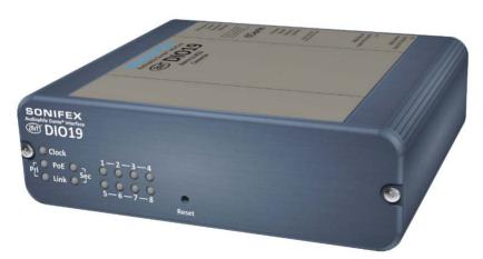
The AVN-DIO19 audio converter and interface converts up to eight digital stereo AES3 inputs and eight digital stereo AES3 outputs to and from the Dante Audio-over-IP networking standard. Each input can accept sample rates from 32kHz to 192kHz, which will be sample rate converted to the Dante system sample rate. All outputs follow the Dante system sample rate.
