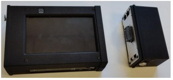
Picture 2: Codec + battery bloc split off
