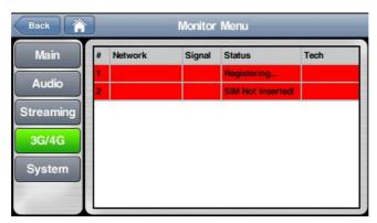
Picture 10: Red colour indicates the network access is not ready yet.
