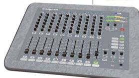
**S1:** The Sonifex S1 mixer is a high performance compact, low-cost, fixed format mixing console designed for on-air radio use. It can be fitted flush into a desktop or rack mounted by the addition of rack ears. It has 10 dual input channels consisting of four mono mic/line inputs, one telco/line input, one stereo cleanfeed/stereo line input, three dual stereo line inputs and
