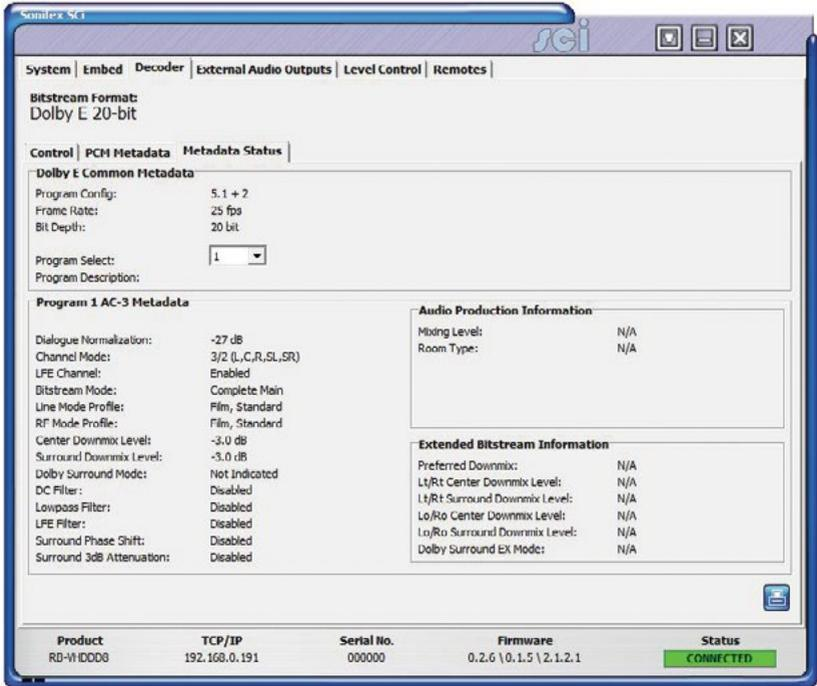
Fig 2-10: RB-VHDD8 Decoder Metadata Status Screen.
