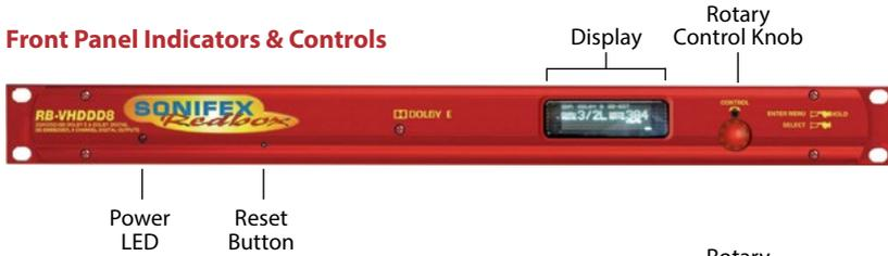
Fig 1-5: RB-VHDDD8 Front Panel Indicators & Controls.
