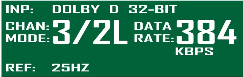
Fig 1-11: RB-VHDDD8 Dolby Decoder Status Screen when decoding Dolby Digital.
