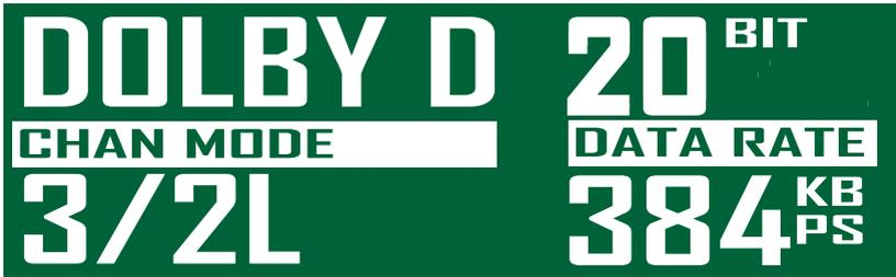
Fig 1-12: RB-DEED8 Decoder Status Screen when decoding Dolby Digital.
