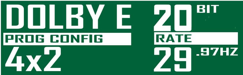
Fig 1-11 RB-DEED8 Dolby Decoder Status Screen when decoding Dolby E.
