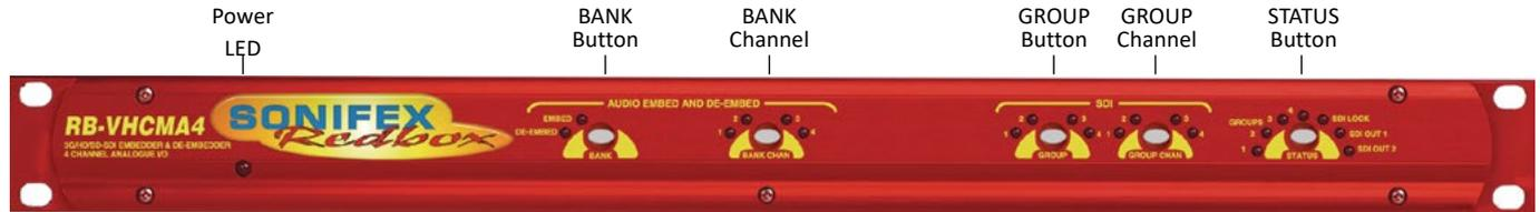
Fig 6-2: RB-VHCMA4 Front Panel
