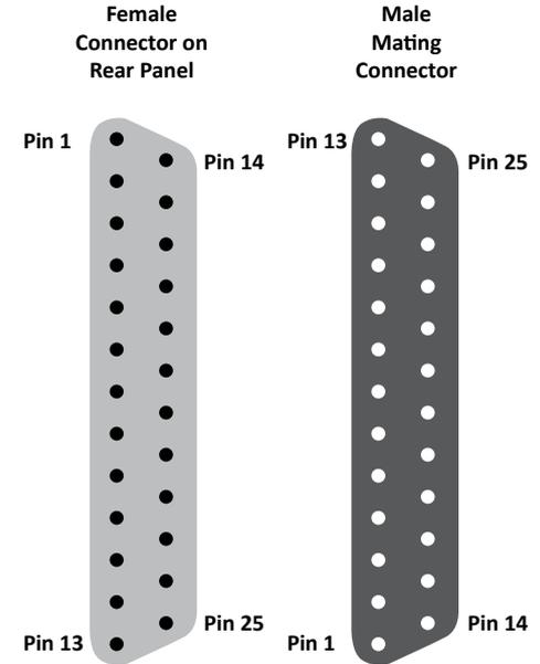
Fig 6-5: The RB-FS82 Female and Male Connectors
