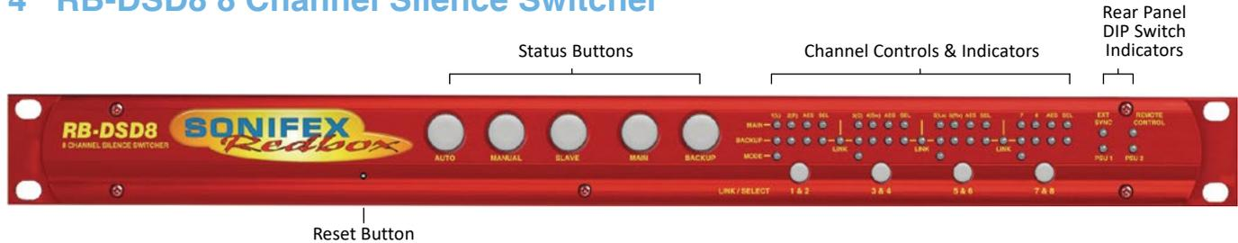
Fig 4-1: RB-DSD8 Front Panel
