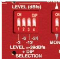
Fig 3-5: SILENCE Detect Audio Trigger Level DIP Switch
