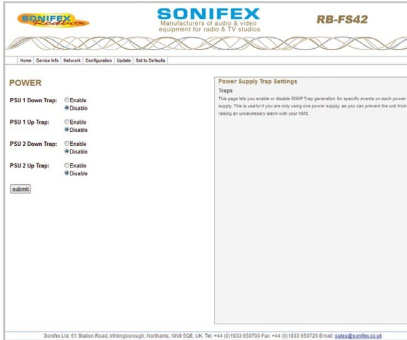
Fig 5-13: The RB-FS42 Power Supply Trap Settings Screen
