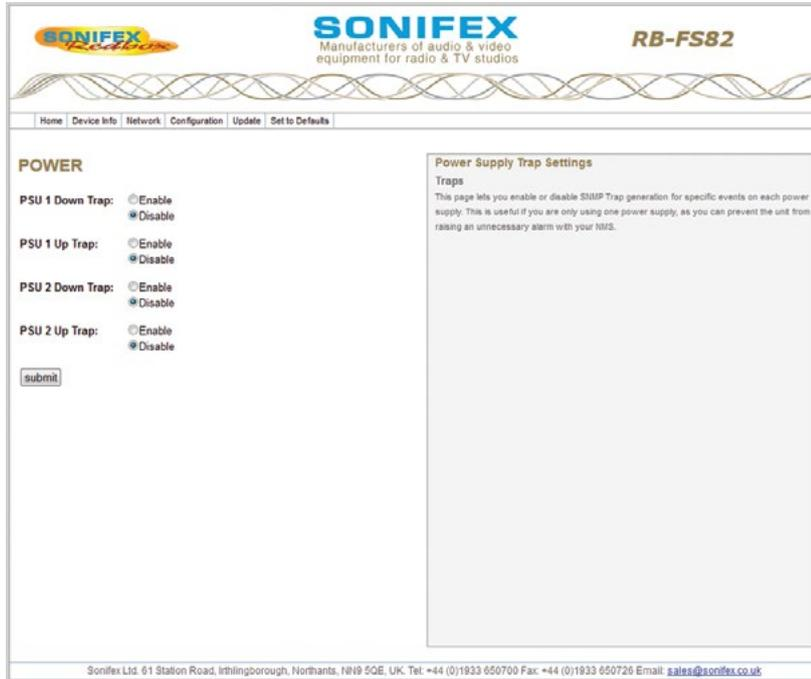
Fig 6-13: The RB-FS82 Power Supply Trap Settings Screen
