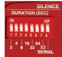
Fig 3-4: SILENCE Detect Duration DIP Switch
