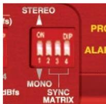
Fig 3-6: SILENCE Detect Stereo/Mono & Sync Source DIP Switch
