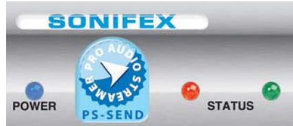
Fig 2-2: PS-SEND Power & Status LEDs
