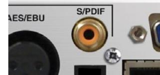
Fig 2-9: PS-SEND S/PDIF Input
