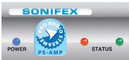
Fig 3-2: PS-PLAY Power & Status LEDs
