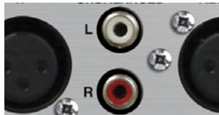
Fig 2-7: PS-SEND RCA Phono Analogue Inputs
