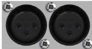
Fig 2-6: PS-SEND XLR Analogue Inputs
