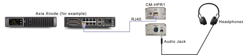
Fig 1-3: Application Example Using Axia Xnode
