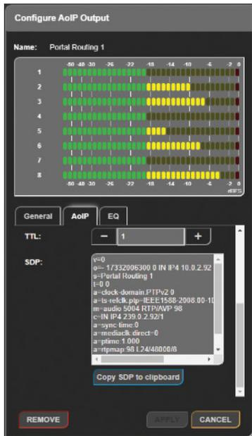
Fig 8-21: AoIP Tab of Configure AoIP Output Window
