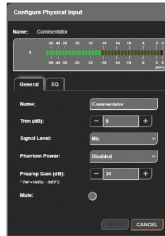
Fig 8-27: General Tab of Configure Physical Input Window (AVN-PM8) - Mic Level
