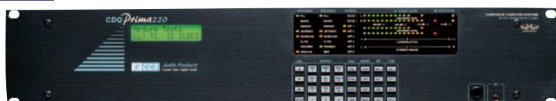
Ideal for attended operations and studio remotes with connection to up to three ISDN BRIs. Includes VU meters, status LEDs, AES/EBU I/O, headphone and front panel R/C jacks, RS485 port - 3x interface module slots.
