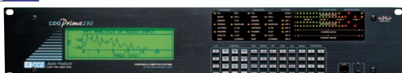
Our deluxe model, for studio head end use and critical monitoring locations. Includes all features listed above, plus graphics LCD, spectrum analyzer, X-Y phase display, extended keypad with assignable hot keys and enhanced status display – 3x interface module slots.
