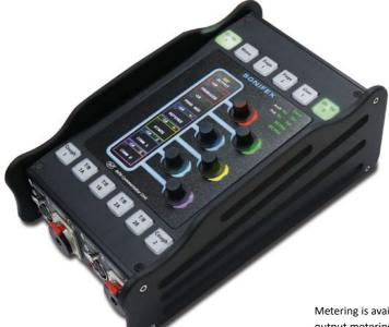
The 6 x push-button rotary encoders and 12 x key-cap buttons are fully configurable, to control input & output levels and panning.
