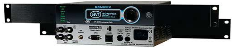
AVN-GMCS IEEE1588 PTP Grandmaster Clock with GPS Receiver
