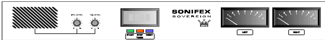
Fig 8-1 : MX10 Meter-Bridge with PPM's
