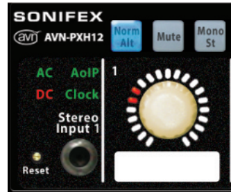
Fig 2-3: AVN-PXH12 Status Indicators & Front Panel Controls
