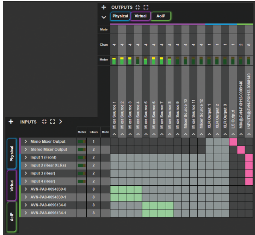
Fig 4-3: The Audio Routing Grid on the ‘Audio Routing’ Web Page
